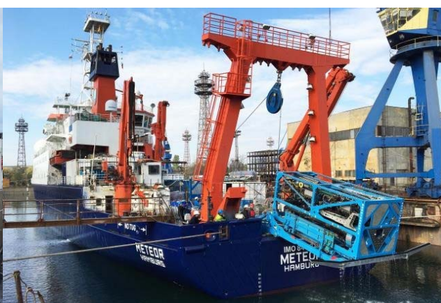
Figure 2: RV METEOR with her new color in the flooded dock of Odessos Shipyard. After installation of MeBo200 on the working deck, the MeBo functions were tested in the dock, among others the drill rig was launched in the water.
