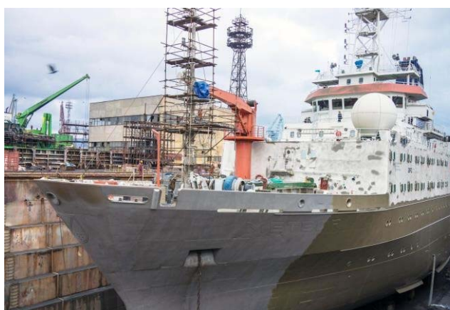
Figure 1: Research vessel METEOR in dry-dock at shipyard in Varna. After cleaning the ship's hull by sandblasting down to the pure steel, the new bronze grounding was applied. (© Heike Dugge).
