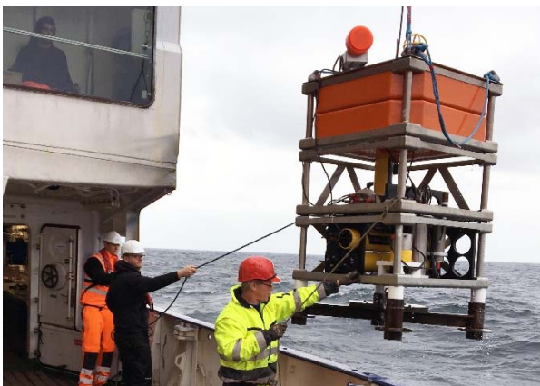
Figure 1: The gas lander during launching procedure from the ship. Before its operation it has to undergo a floating test.
