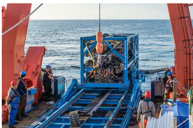
Figure 1: MeBo200 being launched via the A-frame of METEOR. The modern launching-system enables a safe launching of this large device. (© C. Rohleder).
