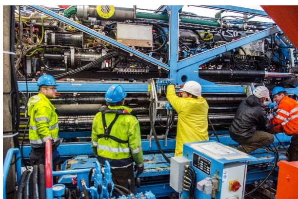
Figure 3: Side view of MeBo200 after the first drilling during cruise M142. Taking the core tubes out of the magazines by means of a special construction, a hydraulic loading/unloading unit. (© P. Wintersteller).
