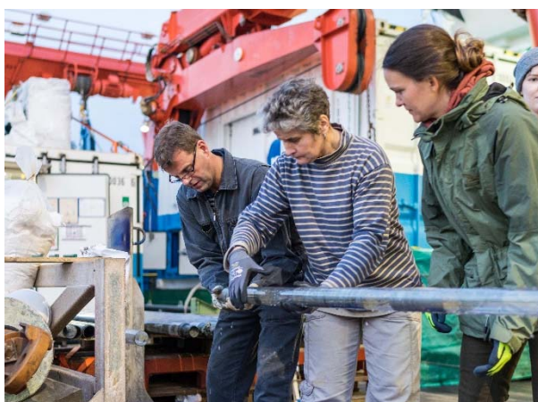
Fig. 1: MeBo200 sediment core had just been pulled out of the core barrel by the scientists and is carried to the lab for further treatment (© C. Rohleder).
