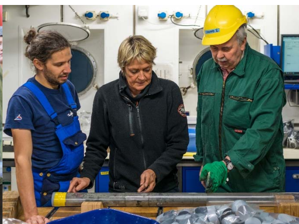
Fig. 2: In the Geo lab the 3.8m long sediment core being cut into shorter segments and labeled before being longitudinally cut in archive- and work half (© C. Rohleder).
