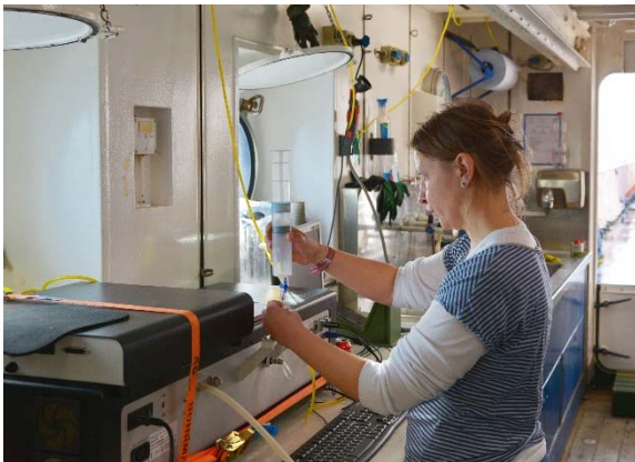
Fig. 1: Dr. Susan Mau in GEO-lab aboard METEOR, measuring greenhouse gases CO 2 und CH 4 in air and water by means of a Laser-based ICOS device. (© A. Popa).
