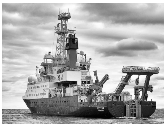
Fig 3: While the drill rig is in action, the vessel stays on the same position for 2-4 days. Only the cable, which is managed via the A-frame into the water and the launching system of MeBo is visible (© M. Beims).
