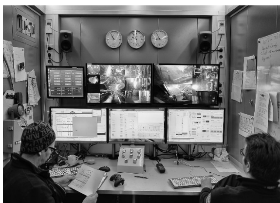
Fig 1: Two operators control the MeBo system from the control container. By means of data and video transmission from the drill rig, Werner Schmidt und Adrian Stachowski control the drilling procedure at the sea floor (© M. Beims).
