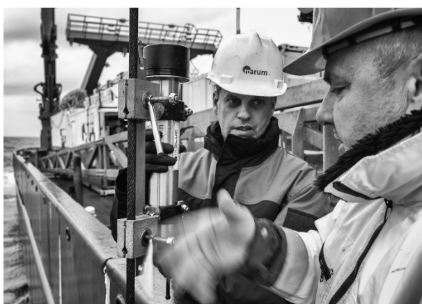
Fig 4: For a precise underwater navigation of positioning all devices on the sea floor, we use the ship's owned Posidonia system. For this, Thomas Pape mounts the Posidonia transponder on the ship's wire above the gravity corer, together with ship's mechanic Henry Schabeck (© M. Beims).
