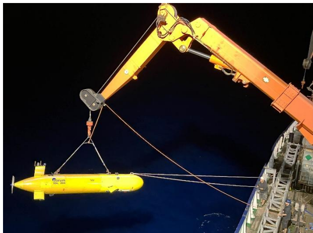
Figure 2: Nighttime deployment of the MARUM AUV using the METEOR's ship crane. The AUV remains in operation for up to twelve hours and is only recovered the following day. (© G. Bohrmann).
