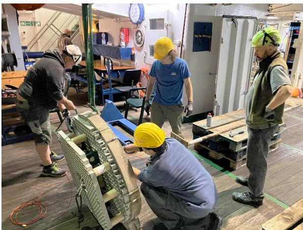
Figure 3: With the support of the team, the scientists assemble the individual components for the in-situ piezometer on the eve of the mission. (© Gerhard Bohrmann).
