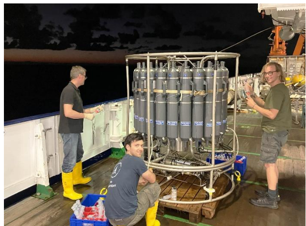
Figure 4: We use the ship's CTD with water samplers almost daily. On our expedition, we primarily measure the methane dissolved in the water. (© Gerhard Bohrmann).
