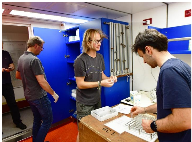
Figure 2: Sample processing in the METEOR chemistry laboratory. After each CTD station, the samples from the 24 water samplers are analyzed for their methane content. (© Elmar Schreiber).
