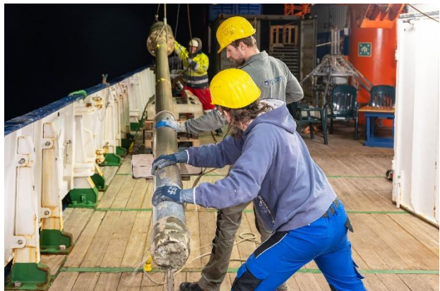
Fig. 4: During the cruise, we extracted 23 sediment cores from the seabed using a gravity corer. The scientists and crew work together to retrieve the gravity corer from the deck, either during the day or at night. (© Andreas Täuber).
