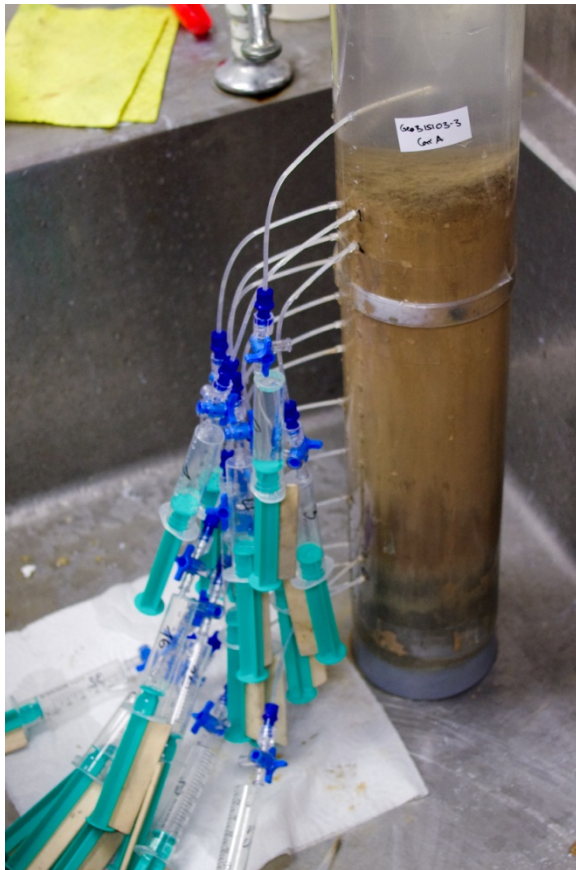
Fig. 1.14. Rhizon pore water sampling from multi-core GeoB15103-3.
