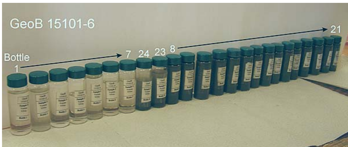
Fig. 1.4 Samples from the water rosette at station GeoB 15101-6. Samples 8-21 (downcast) and 23-24 (upcast) contained suspended mud.
