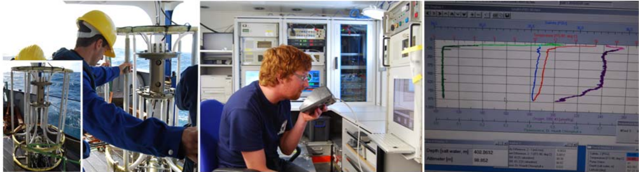
Figure 4.4. Deployment of CTD frame, CTD watch, screen showing fluorescence (green), salinity (blue), temperature (red), and oxygen (purple) data recorded during a CTD cast (from left to right; photos: J. Stone, MARUM).
