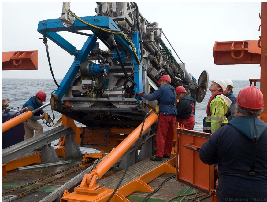
Fig. 1.4 The sea floor drill rig MeBo during deployment from R/V METEOR.
