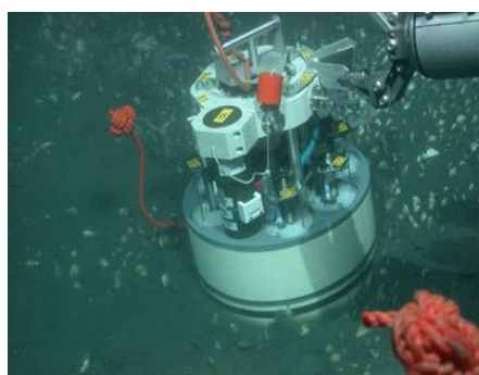
Fig. 4.3 Respiration measurements with the benthic chamber
