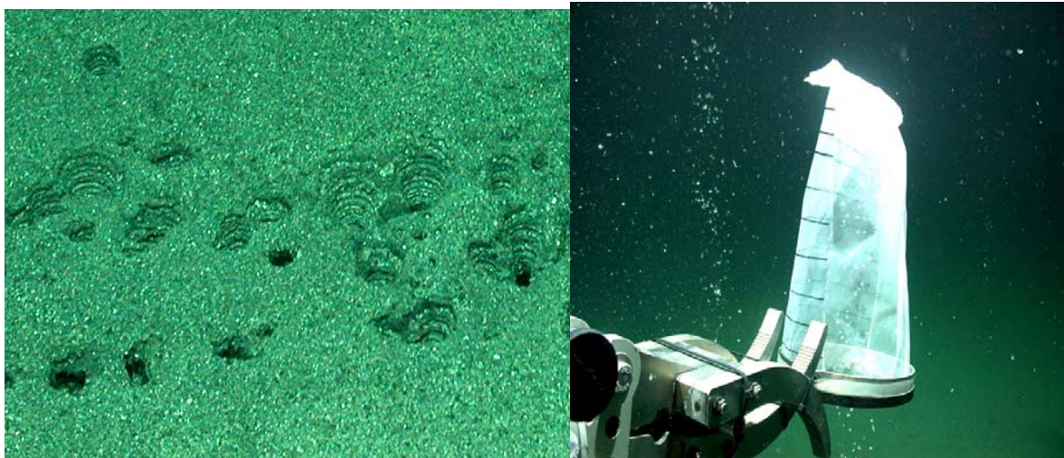
Abbildung 2: Single bubble streams emanating from the seafloor leave individual holes in the seabed in 850 m water depth (left), from which the wall structures document the youngest sediments like the whitish coccolith ooze layers. Right image: One of two bubble streams is caught in plastic bag on the manipulator arm of ROV QUEST. By measuring time and volume a simple quantification of methane release from the seafloor is possible. Images taken by ROV QUEST (MARUM)
