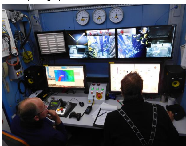
Figure 3: View of the MeBo-control station where the drilling is conducted and progress monitored.
