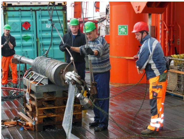
Fig. 1: Deployment of the 3 m long gravity core for sampling of mud breccia.
